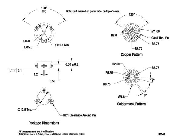
Figure 2. SKYFR-000742 Package Dimensions and PCB Footprint
