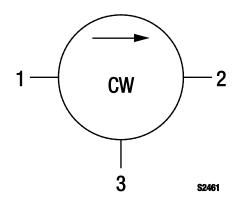
Figure 1. SKYFR-000742 Block Diagram
