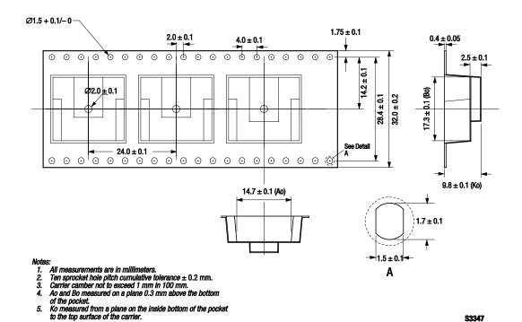
Figure 3. SKYFR-000742 Tape and Reel Dimensions
